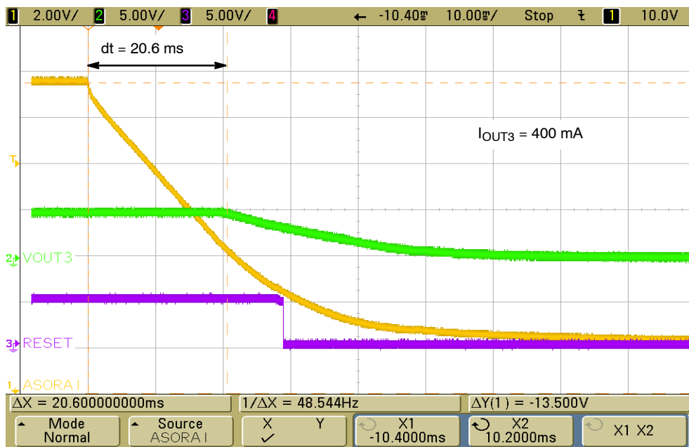
Figure 29. Output Response of LDO3 to Loss of Vin-B
